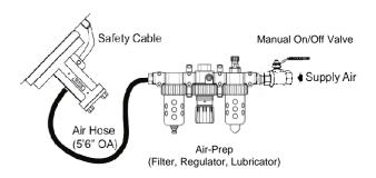
Single-unit manual installation for bins and hoppers is shown here for reference purposes.
