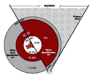
This illustration compares the force output and noise output of QI, IMP, and AC versions of the BV-225 size piston vibrator. See below for complete specifications.
